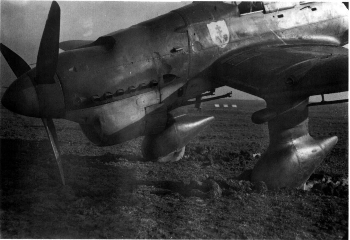
Landing the Stuka was straightforward but required the pilot's full attention, as the aircraft had a tendency to nose over on touchdown. (via Phil Jarrett)
