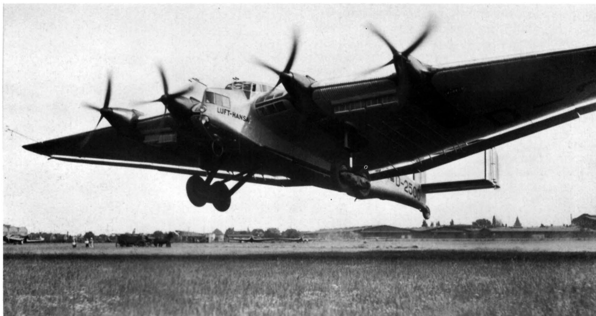
The four-engined Junkers G.38 was the largest commercial aircraft of its time. Note the patent Junkers double-wing ailerons and hydraulically-operated flaps, which were also a feature of the Stuka. ( Lufthansa )
