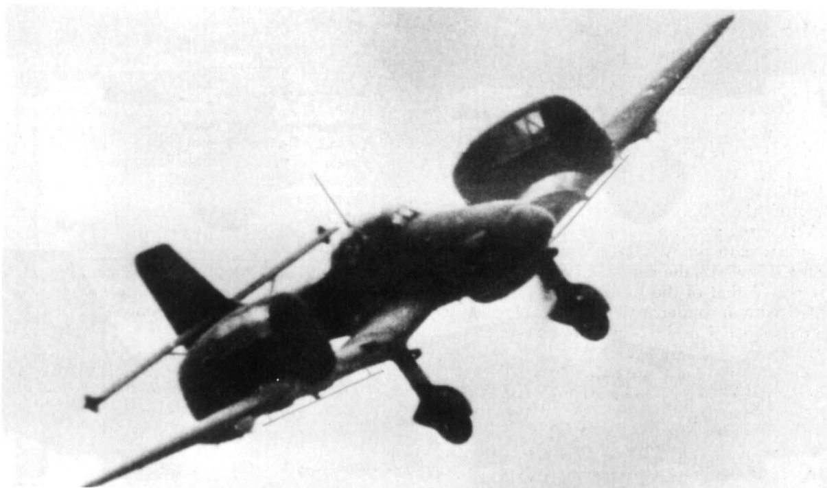
This Junkers Ju 87D-3 was an experimental passenger-carrying variant. It was fitted with wing-mounted personnel pods and tested at the Graf Zeppelin Research Institute at Ruit, near Stuttgart, in 1944. The pods, designed to carry two men each, were non-jettisonable. (via Phil Jarrett)
