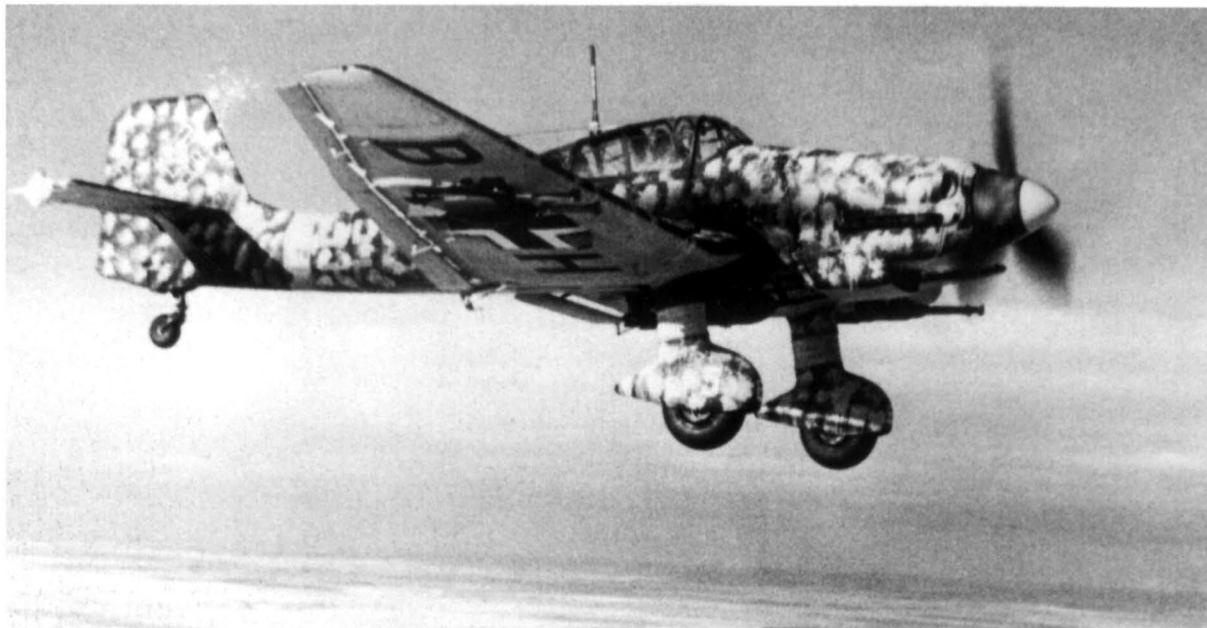
A Ju 87D-5 over Russia, 1944. The aircraft's national markings have been obliterated by the temporary 'snow camouflage', which was hastily applied with the onset of winter. (via Phil Jarrett)
