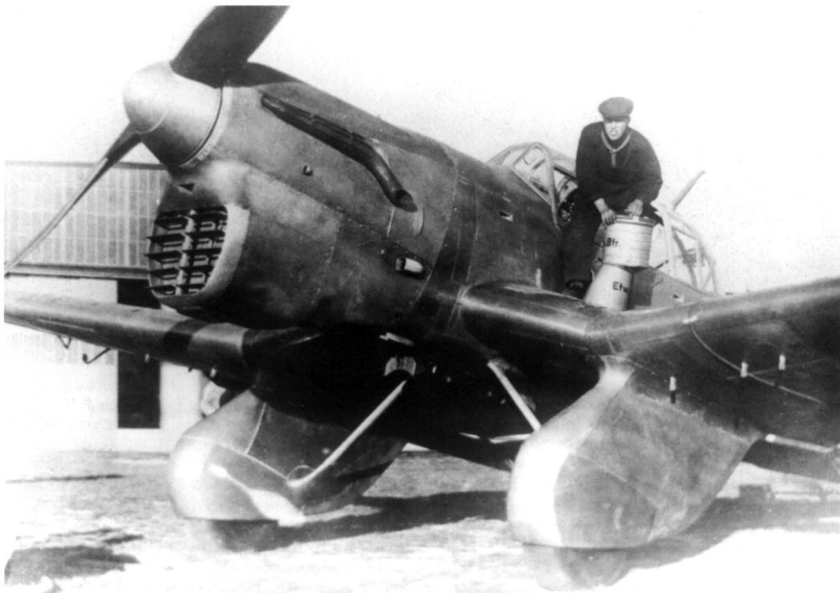
The Ju 87V-1 prototype being refuelled at Dessau during the autumn of 1935. The dive brakes have not yet been fitted, although their mountings are visible. (via Phil Jarrett)
