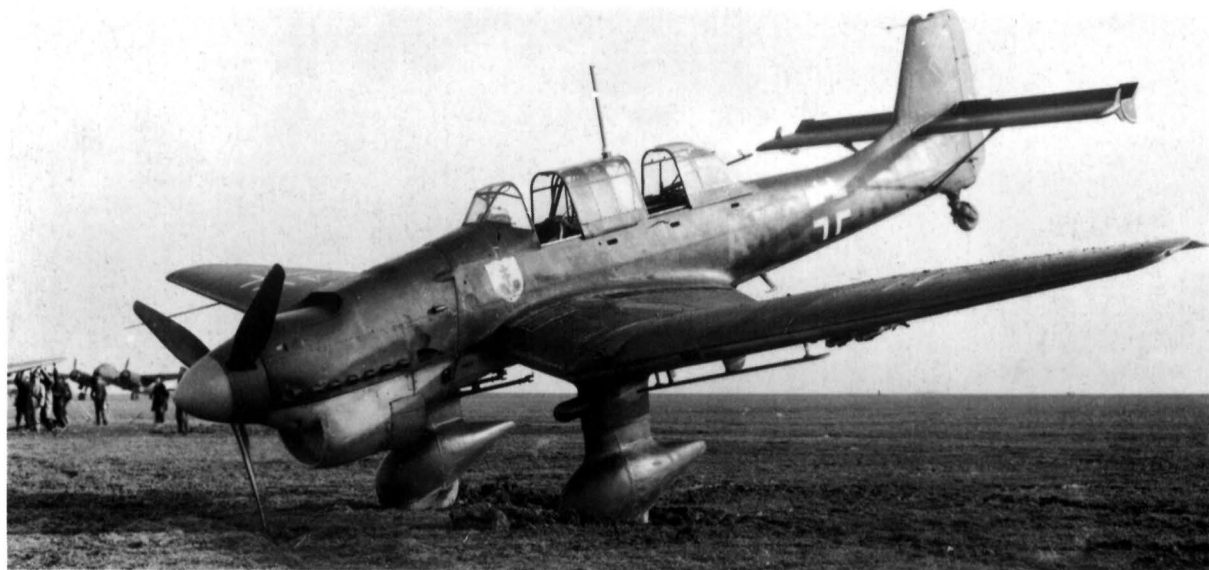
Ju 87B-2 NO+HP of III/StG 2 seen after nosing over on muddy ground at Prague-Ruzyně in November 1941. The Stuka was prone to such unwanted manoeuvres if its pilots did not take care. (via Phil Jarrett)
