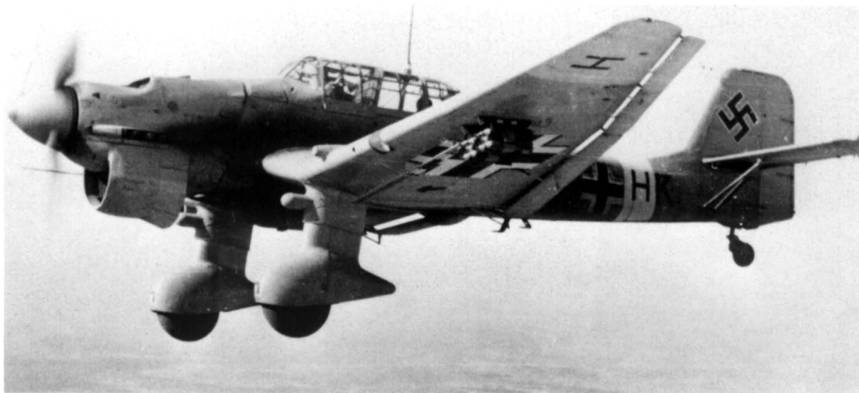
A Ju 87D carrying a cluster of fragmentation bombs under each wing. Stukas carrying such armament were deadly weapons against troop concentrations and unarmoured vehicles. (via Phil Jarrett)
