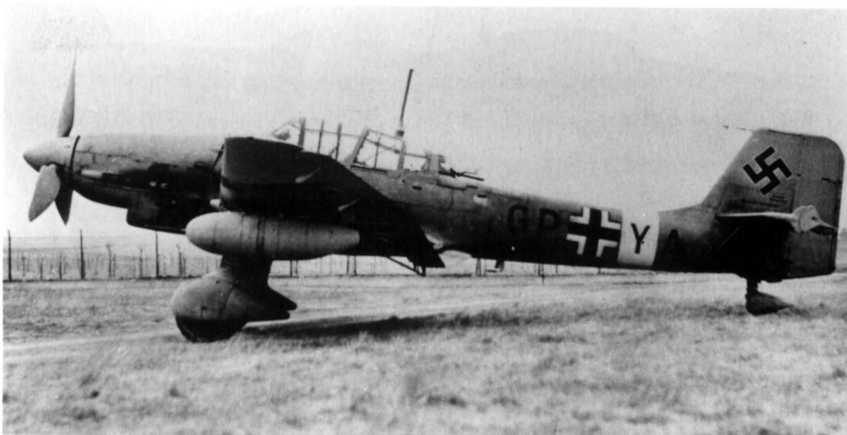
A Ju 87D-1 (Trop) with 66 Imp gal underwing fuel tanks. Note the large paddle-blade propeller. (via Phil Jarrett)
