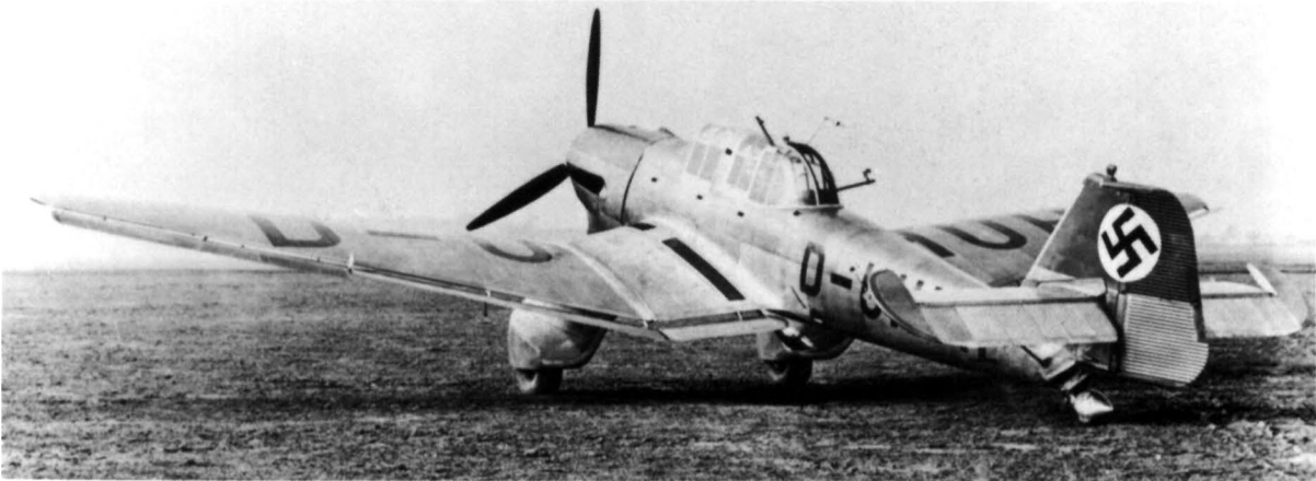
The second prototype Junkers Ju 87V-2, D-UHUU, was powered by a 610-hp Junkers Jumo 210A engine. It featured a single fin and rudder, a modification incorporated after the loss of the Ju 87V-1. (via Phil Jarrett)
